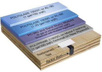
Plywood Substrate System with Rubber Aggregate
