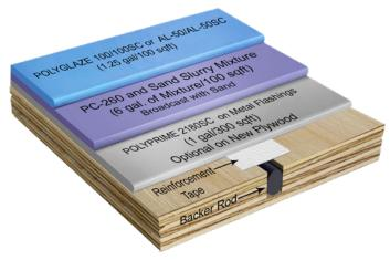
Plywood Substrate System with Sand Aggregate
