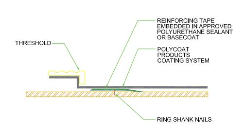
19A SLIDING DOOR THRESHOLD FOR CONCRETE SUBSTRATE
