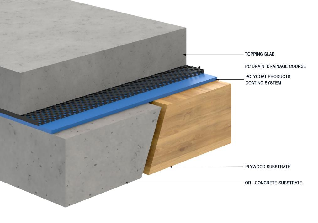
22- BETWEEN SLAB WATERPROOFING
