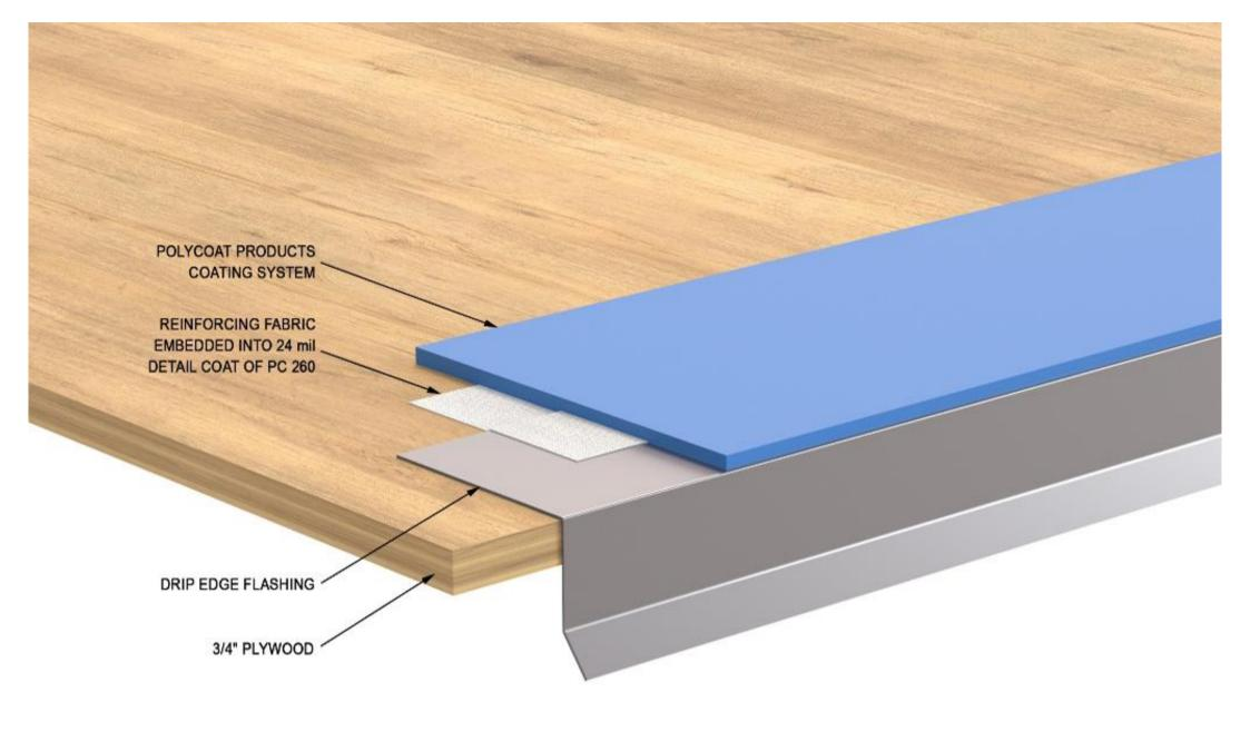
4- OUTER EDGE METAL (See detail 5 for flashing at wall)
