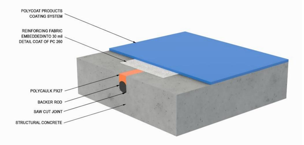
6- SAW CUT CONTROL (New Construction)
